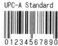
UPC-A Barcode wit Guard Bars Extended 2 mm
